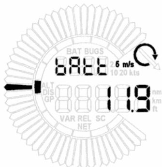
Fig. 30 Battery voltage display
